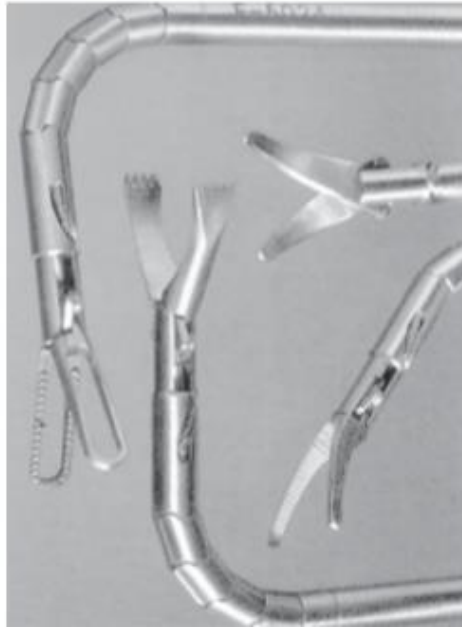
Figure. Laparoscopy tools. The actions of grippers, scissors, tongs and other mechanisms are performed by SMA.
